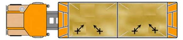
FIGURE 2.4B – DUAL HOPPER-BOTTOM TRAILER, SINGLE-SIDE SAMPLING
