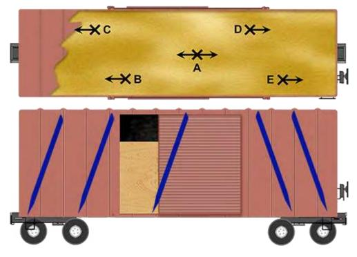
FIGURE 2.2 – BOXCAR, TRUCK, OR TRAILER SAMPLING PATTERN
