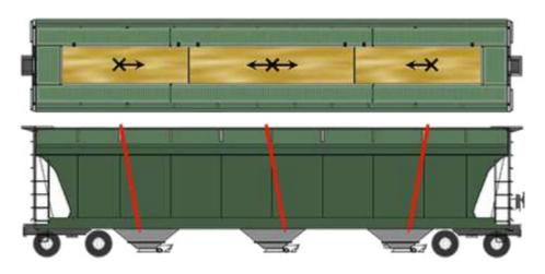
FIGURE 2.1 – HOPPER CAR SAMPLING PATTERN
