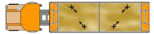
FIGURE 2.4A – DUAL HOPPER-BOTTOM TRAILER SAMPLING PATTERN
