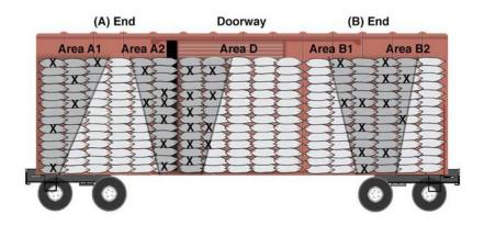
FIGURE 2.2 – SIDE VIEW OF A BOXCAR WITH THREE WELLS, SELECTED BAGS INDICATED BY X MARKS
