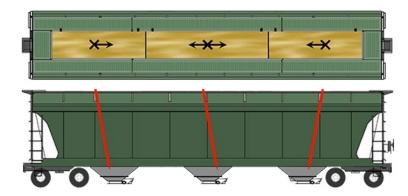
FIGURE 2.4 – 3-COMPARTMENT, TROUGH OR DOOR TYPE HOPPER CAR
