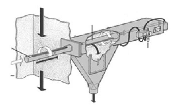
Figure 2. Point-Type Sampler
