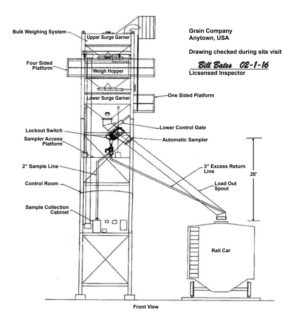
FIGURE 3.1 - DIVERTER-TYPE SAMPLER SITE DRAWING
