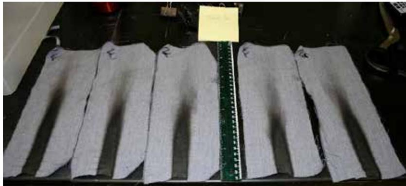
optimum flame resistance performance. 34 blend samples in a woven construction were produced and evaluated for flame resistance and mechanical properties. From this analysis 7 blends are selected and spinning of yarns has commenced.
