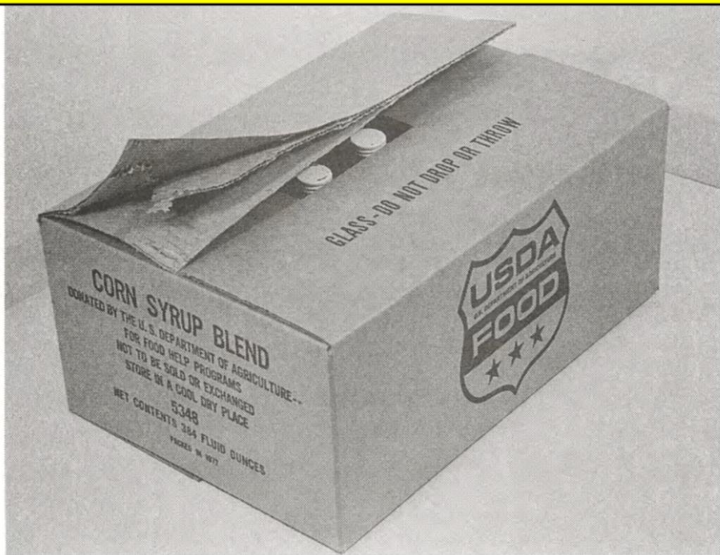
Defect No. 106. Product Sifting or Leaking. Major defect. This primary container allowed the product to sift.
