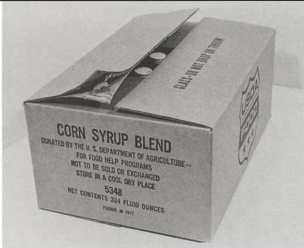
Defect No. 105. Separation of Lamination (Corrugated Fiberboard). Major defect. The lamination is separated in this container to the extent that it affects usability.
