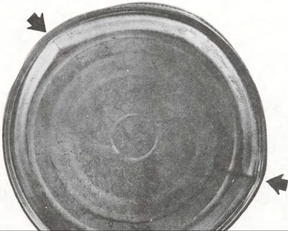
Defect No. 111. Buckle. Major Defect. A permanent distortion of the counter sink (channel next to end seam). Caused by excessive internal pressures developed during processing. The distortion of the end seam is readily noticeable at first glance. There is some suspicion that the end seam has been placed under tension sufficient to jeopardize the hermetic seal.
