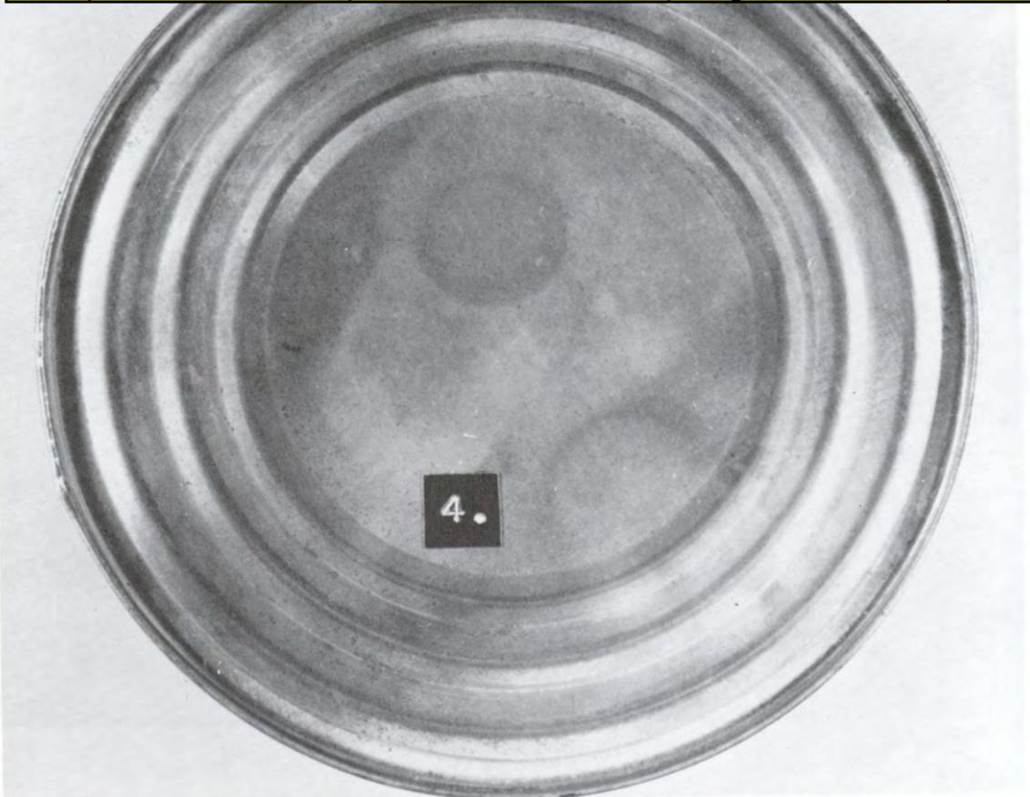
Defect No. 202. Outside Tinplate or Coating (When Required).
