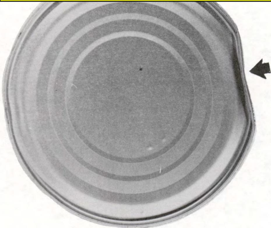
Defect No. 208. Dent. Upper limit of a minor defect. Moderately deep dent on the end seam forcing it inward to such an extent that the counter sink (channel next to end seam) and body are involved, but no sharp ridges are evident.
