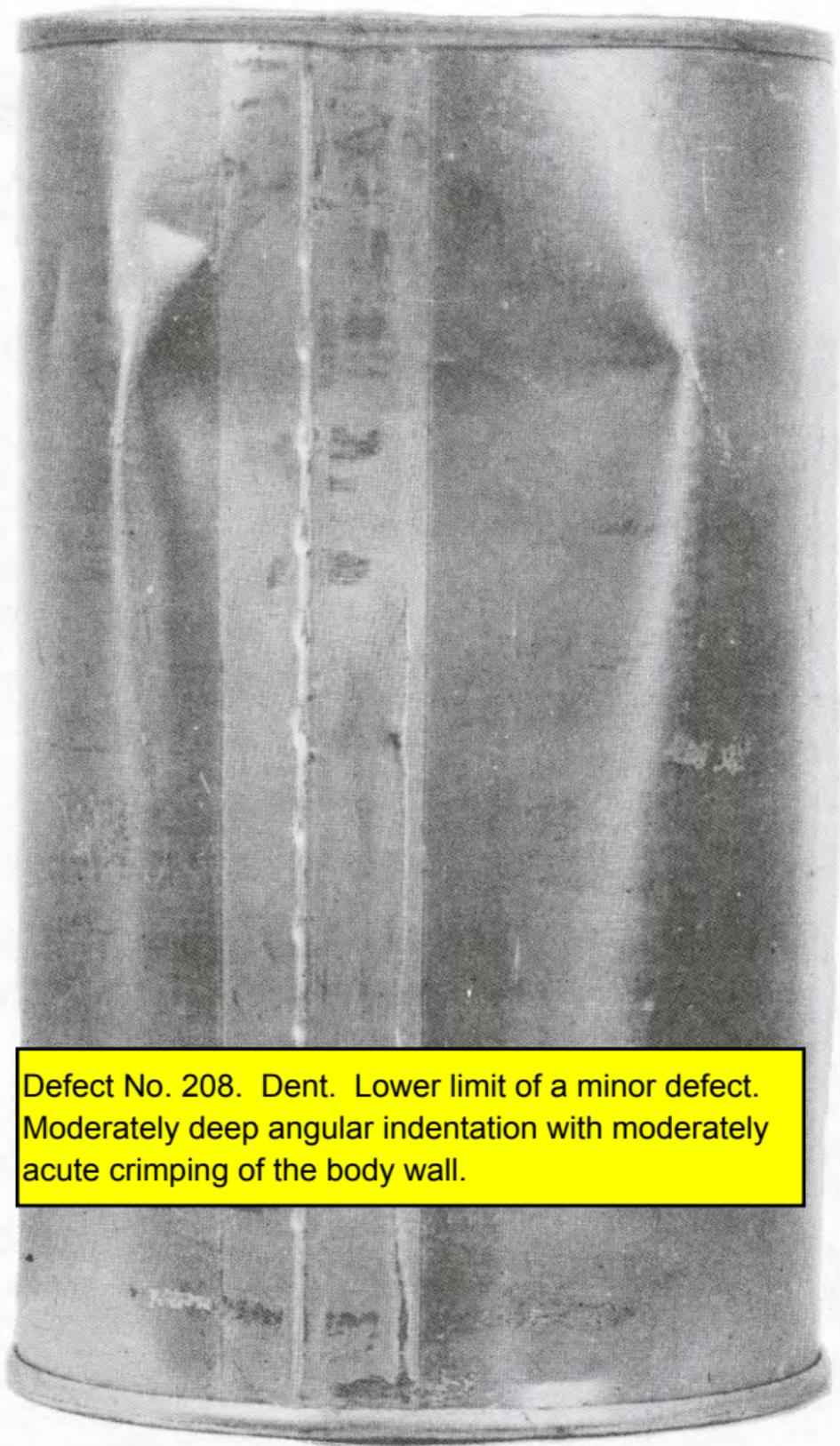
Defect No. 208. Dent. Lower limit of a minor defect. Moderately deep angular indentation with moderately acute crimping of the body wall.
