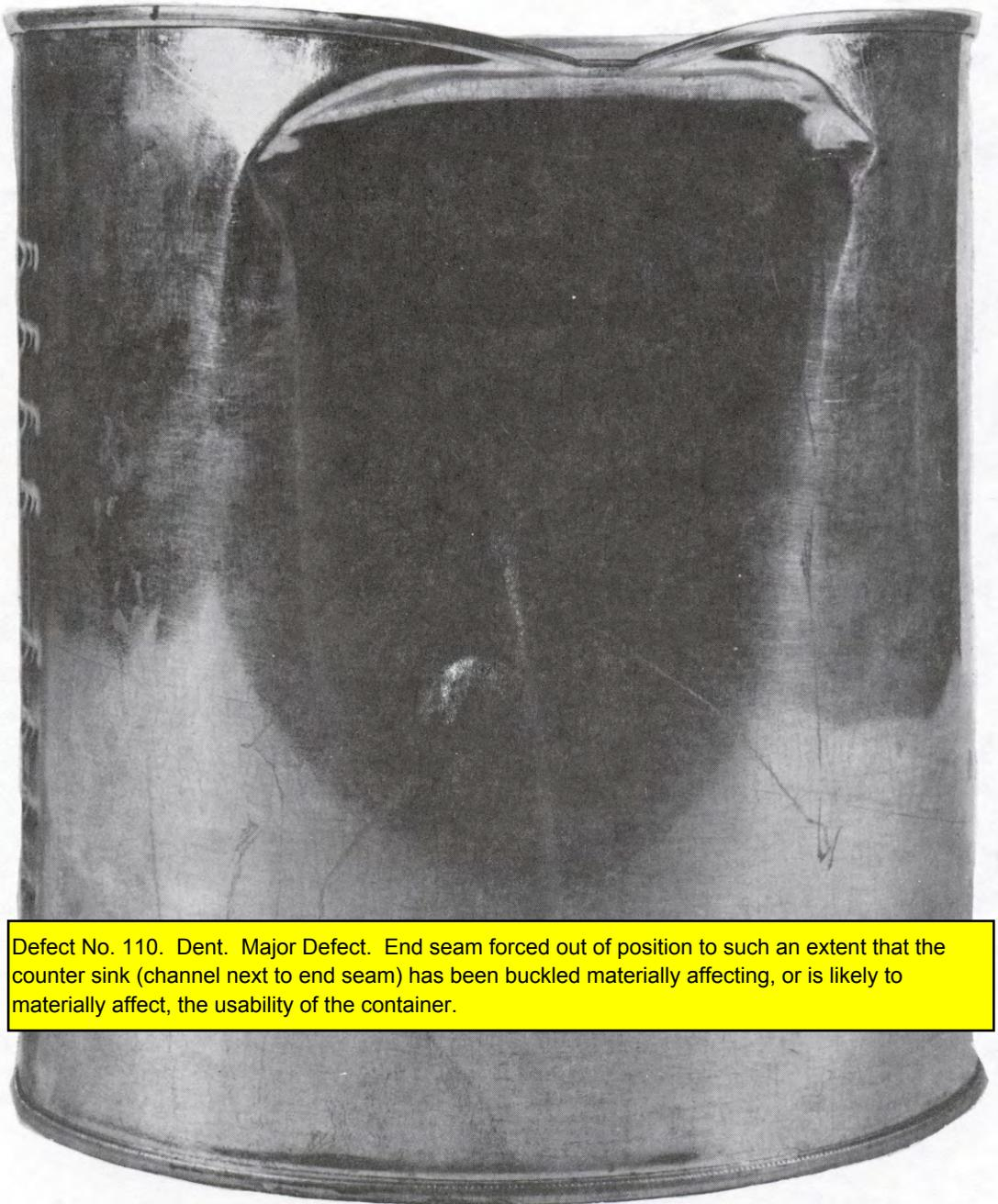
Defect No. 110. Dent. Major Defect. End seam forced out of position to such an extent that the counter sink (channel next to end seam) has been buckled materially affecting, or is likely to materially affect, the usability of the container.
