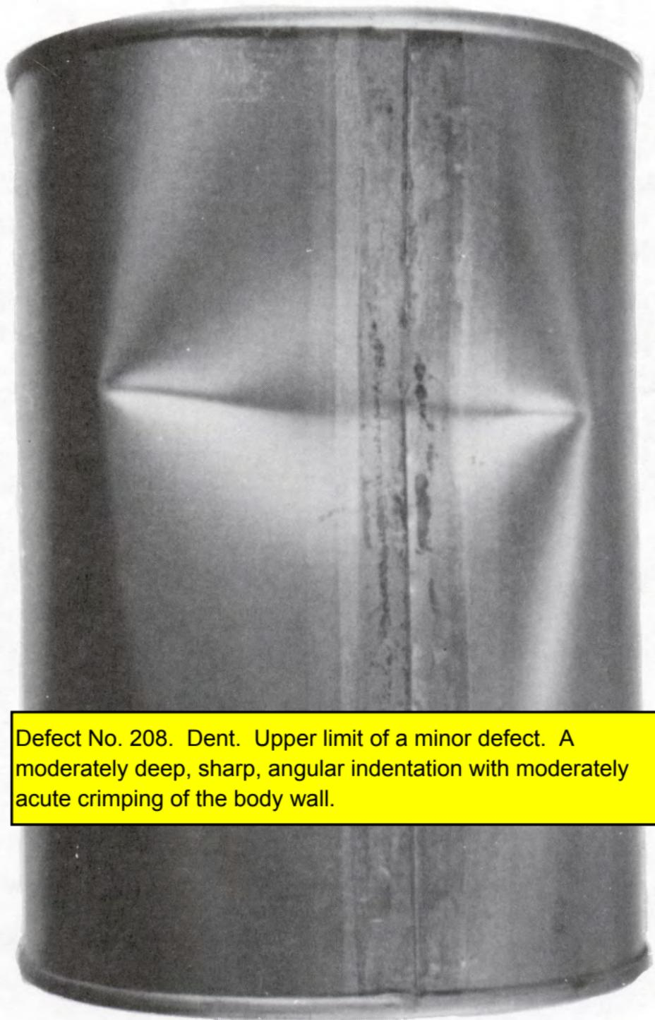
Defect No. 208. Dent. Upper limit of a minor defect. A moderately deep, sharp, angular indentation with moderately acute crimping of the body wall.
