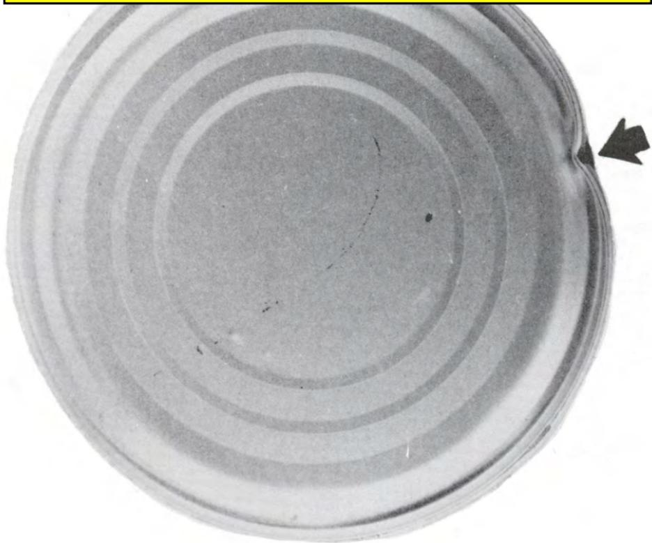
Defect No. 208. Dent. Minor defect. Dent on the end seam forcing it inward to such an extent that the counter sink (channel next to end seam) and body are involved, but not sharp ridges are evident.
