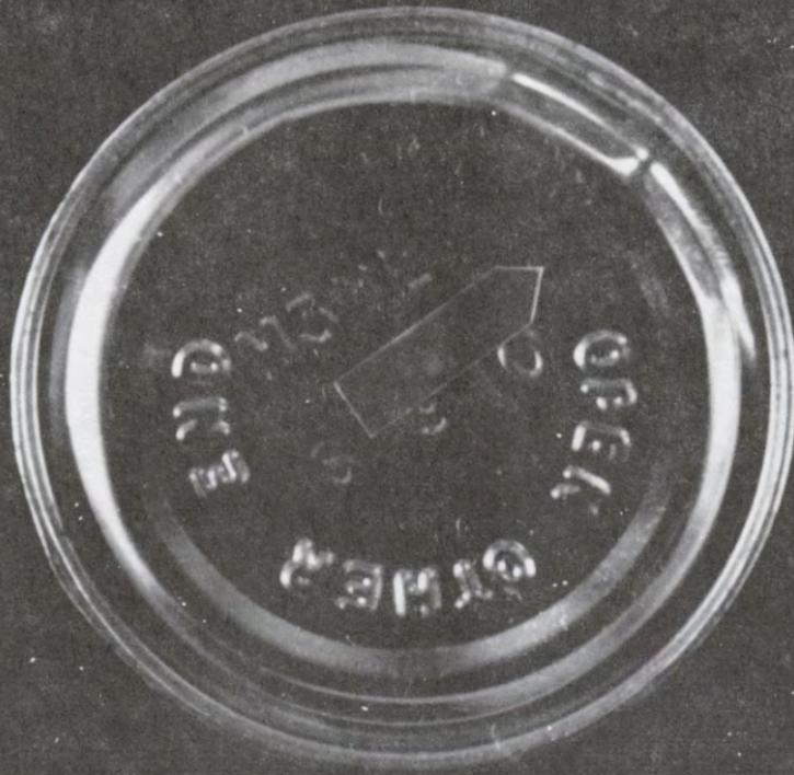
Defect No. 111. Buckle. Major Defect. Buckle barely extending into side seam.
