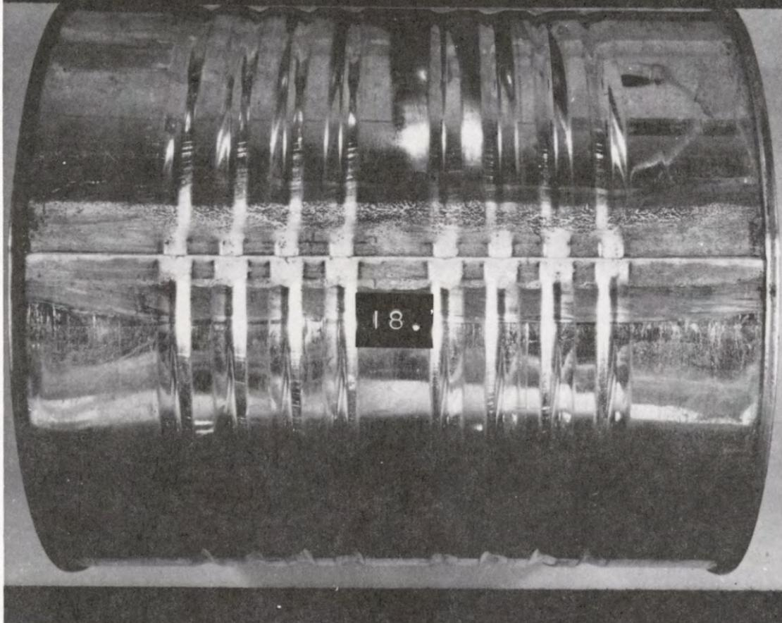
Not a defect. Dirty, Stained, or Smeared. Typical of many well made cans.
