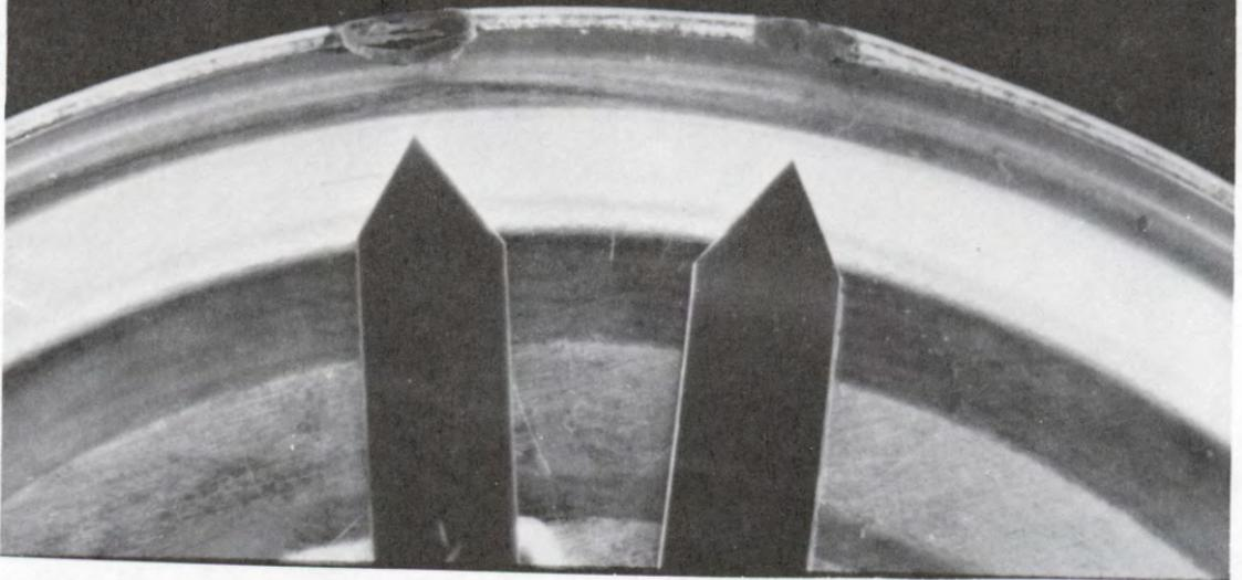
Defect No. 2. Leaker. Critical defect. Leaker caused by severe cable cut. Leakage is evidenced by the corrosive action of an acid product along the lid groove under the cable cut. Score this container once-as a leaker (a critical defect) and not as a cable cut (a major defect). The conditions are related, therefore, the most serious condition is scored.
