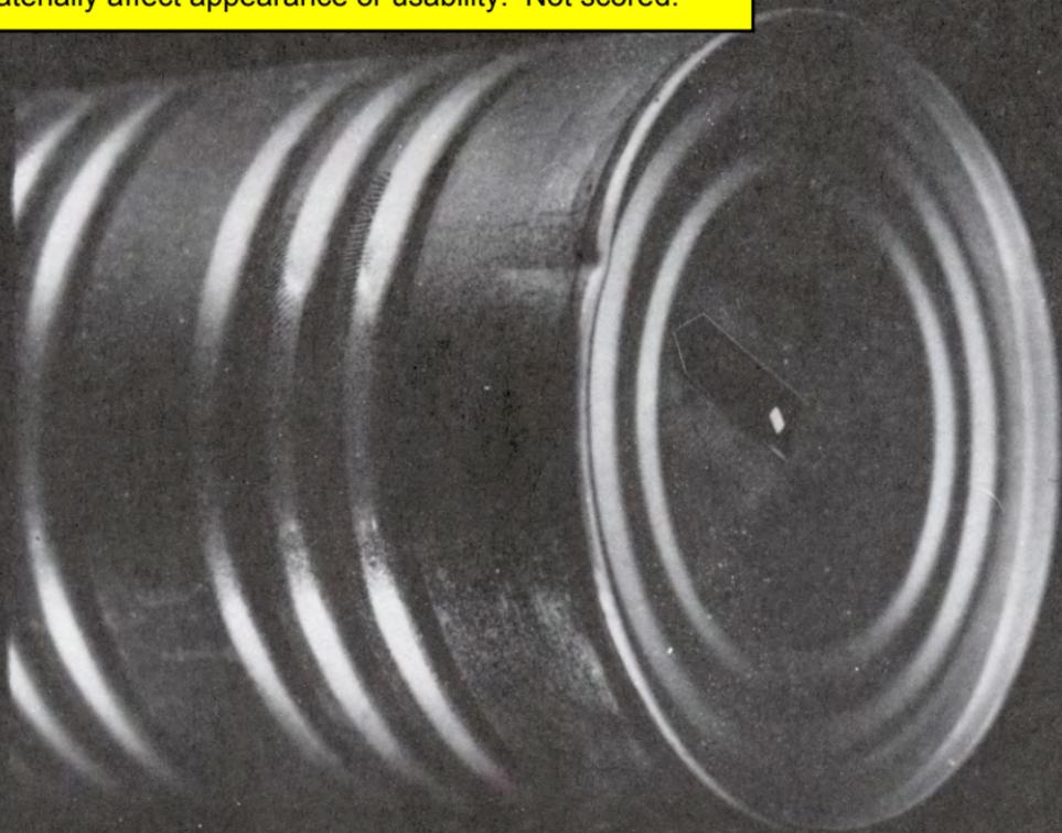
Insignificant defect--not scored. Dent. Not distortion of end seam. Does not materially affect the appearance of usability.
