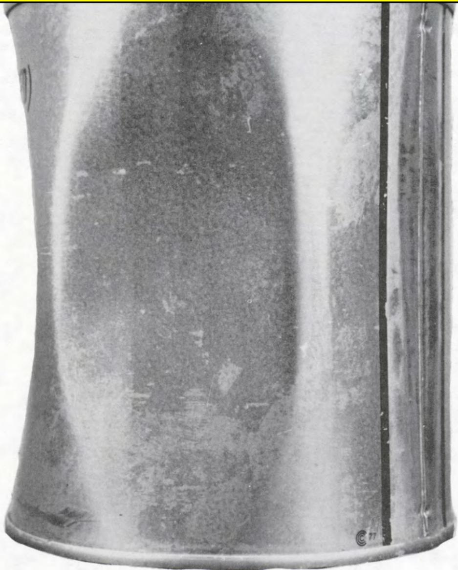
Defect No. 114. Cable Cut. Left pointer. Major defect. Exposed seam laminations. Right pointer. Insignificant defect. Seam laminations not exposed by slight cable cut.
