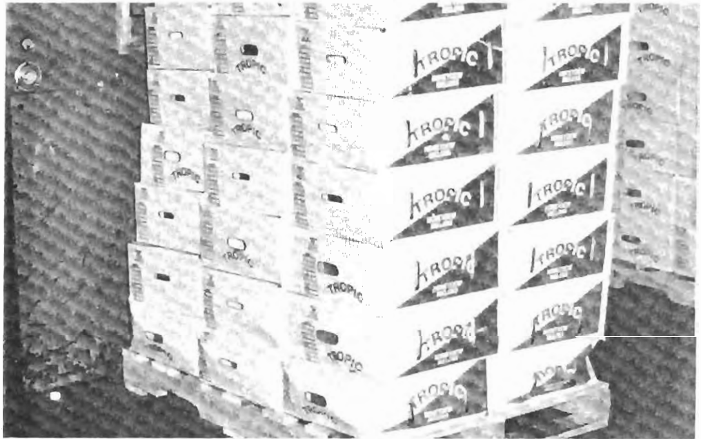
Clear plastic netting helps to stabilize this load of honeydew melons. The boxes are too weak and are not stacked carefully on top of one another. Corners of boxes must align to obtain the maximum box strength.
