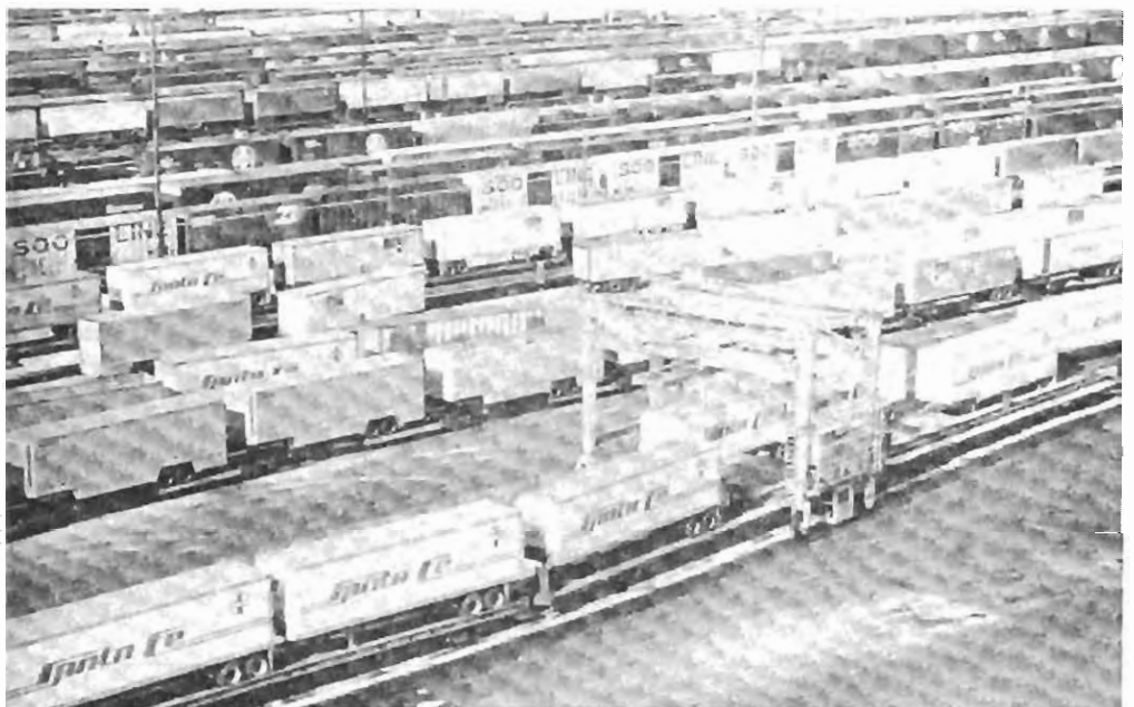
Refrigerated piggyback trailers on railroad flatcars and roll-on/roll-off ocean vessels are used for long distance hauls from California, Florida, Puerto Rico, and Central America. They are driven to and from railroad and ocean terminals to points of origin and destination.
