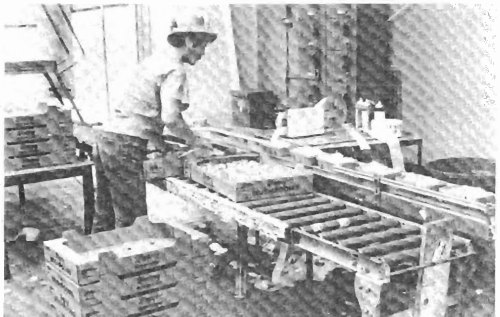
Shed packing of mushrooms in self-locking fiberboard trays. The mushrooms have been prepacked in fiberboard containers, film wrapped, and labeled for retail sale.
