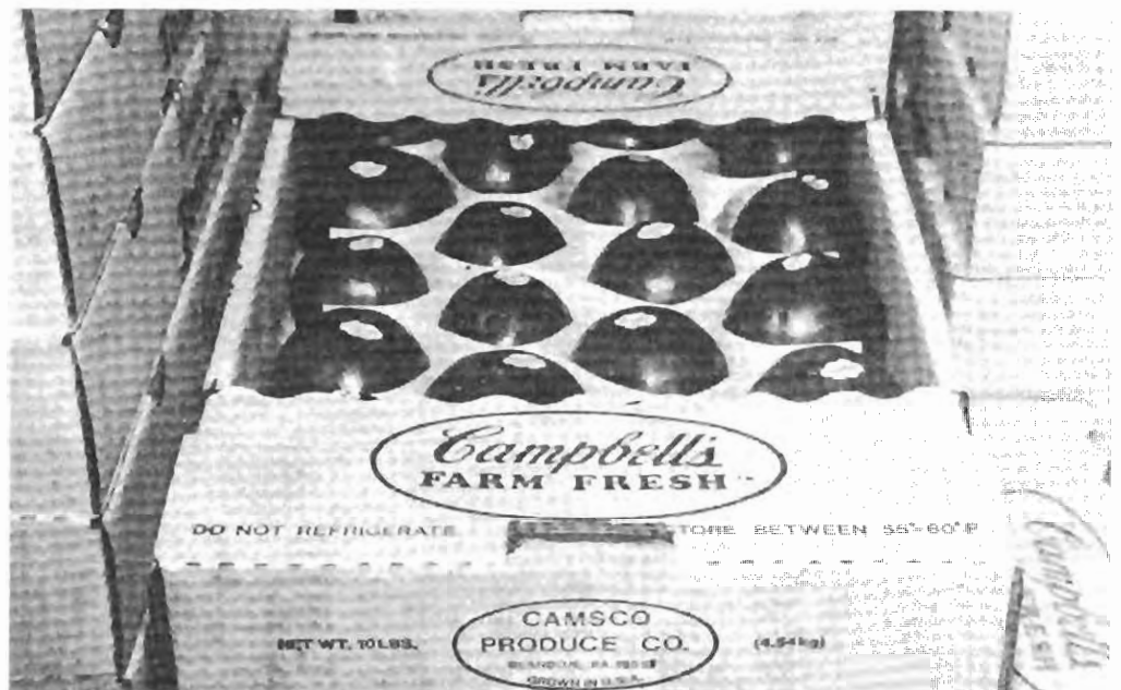
Self-locking fiberboard tray of tomatoes which are protected from bruising by polystyrene foam sheet dividers.
