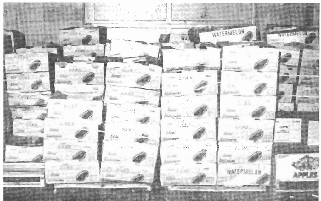
Weak oversized boxes damage these watermelons and make handling and storage difficult. The boxes are very heavy when loaded (34 kg (76 lb)) and they are too wide and too long to be handled carefully. The boxes are too big for a standard pallet, causing pallet overhang and crushing of the box and melons.
