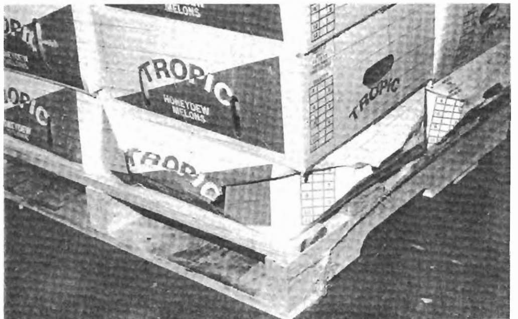
Compression. These melon boxes do not have sufficient strength to withstand multiple handling and the overhead weight of the other containers.
