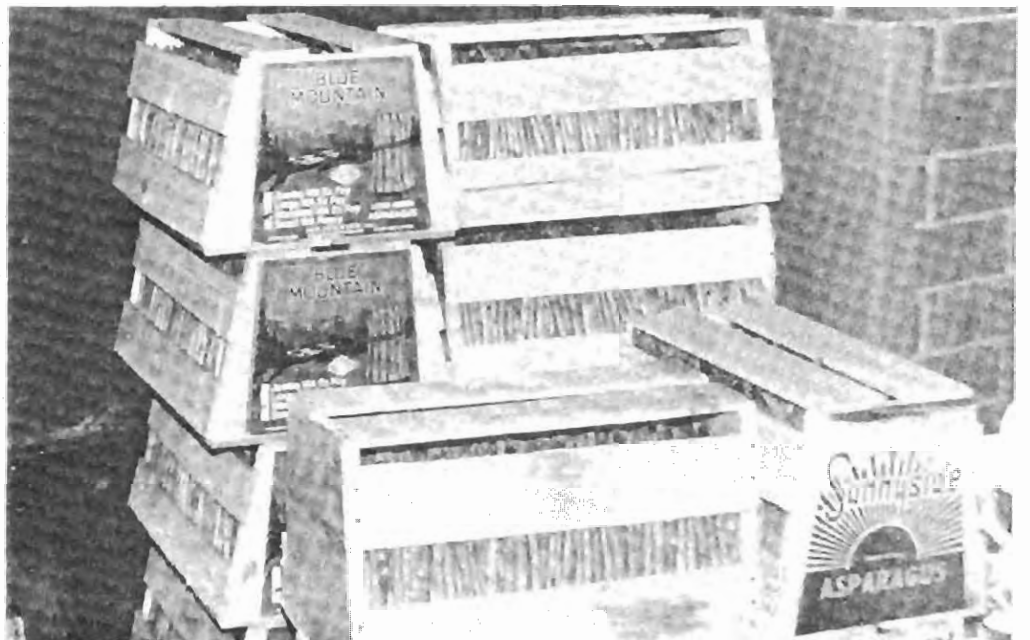
Nailed wood pyramid crates of asparagus. The crates provide compression strength and ventilation. A moistened pad is placed at the bottom of the asparagus stalks to maintain quality.
