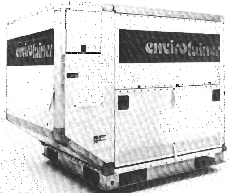
A refrigerated LD-3 air cargo container with a compartment for dry ice on the upper left hand side.
