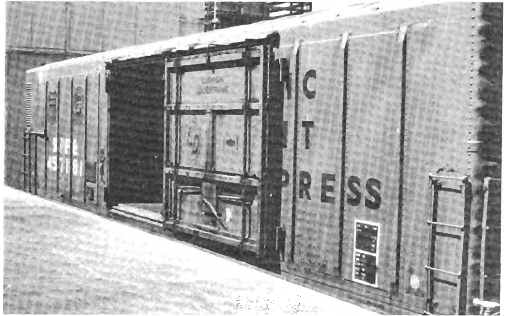
This 18.3 m (60 ft) long mechanically refrigerated railroad boxcar is used for apples, carrots, citrus, onions, and potatoes as well as a limited amount of broccoli, celery, lettuce, and tomatoes.
