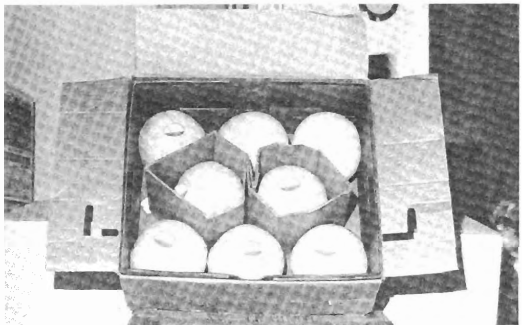
A fiberboard divider adds compression strength to this full telescoping box of honeydew melons with interlocking top flaps.
