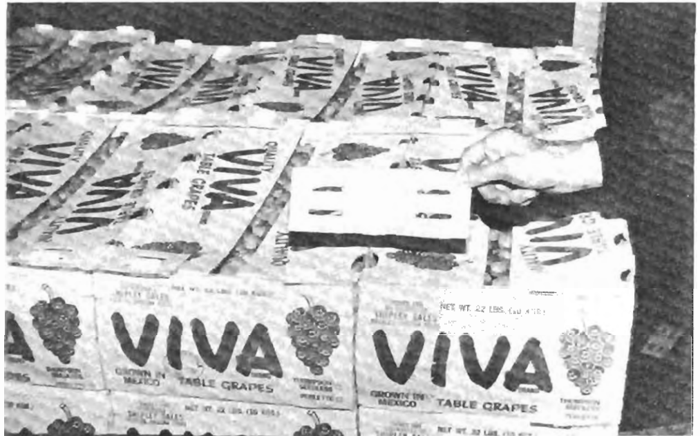
Fiberboard locks between the vertical tabs of each interlocking box of table grapes helps to unitize each layer of boxes horizontally. The plastic end tabs on the boxes unitize the boxes vertically, providing stacking strength and alignment.
