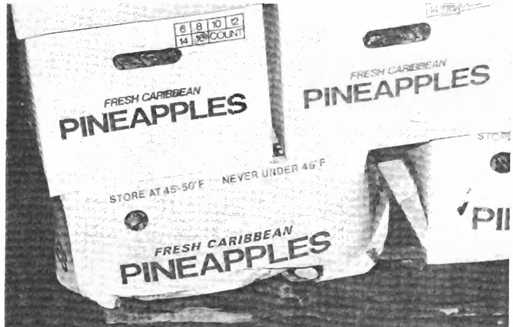
Pallet overhang caused the failure of this pineapple box and damage to the product inside. Boxes lose their compression strength when they are loaded in this manner.
