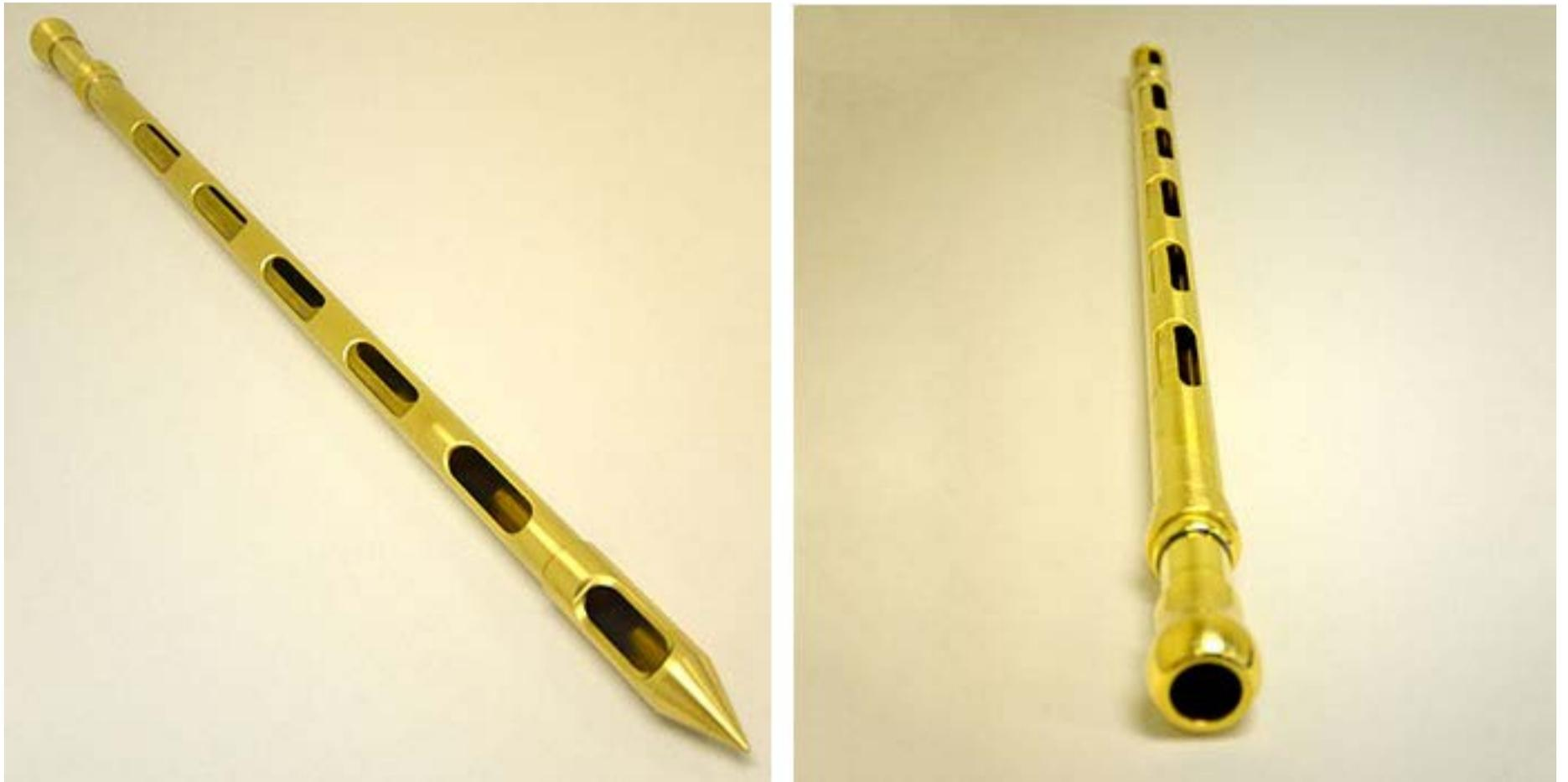
The open-throat probe does not have compartments inside. This feature allows the sample to be poured directly from the probe into a sample container. The open-throat probe tends to draw more grain from the top portion of the lot. Results of the open-throat probe will differ from that of a sample drawn with a compartmented probe.
