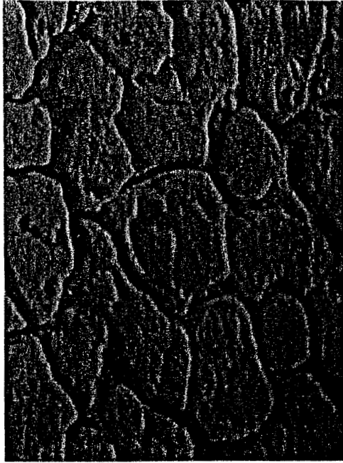
Figure 11. Scanning electron micrograph of the surface of sensitized stainless steel showing preferential attack along the grain boundaries.
