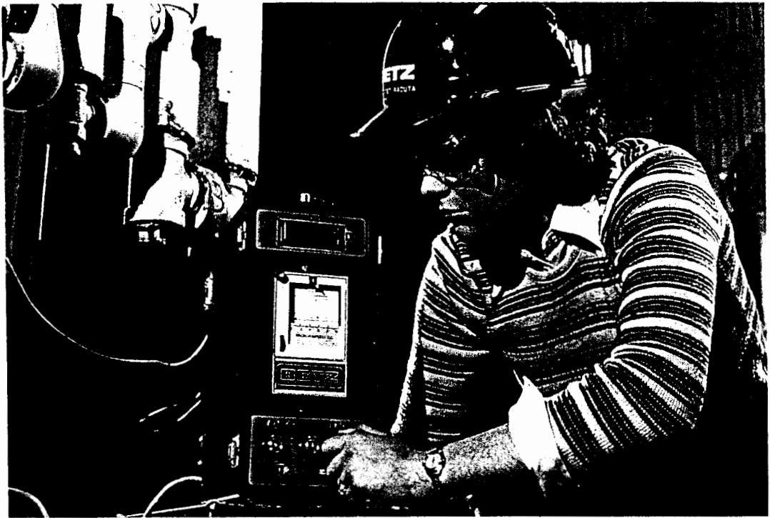
Figure 19-7. Test specimen bypass rack used to monitor amine treatment. Corrosion rate meter on right measures instant corrosiveness values.
