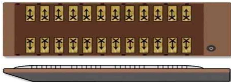
**FIGURE 2.3 – FIBERGLASS HATCH TOP BARGE**
