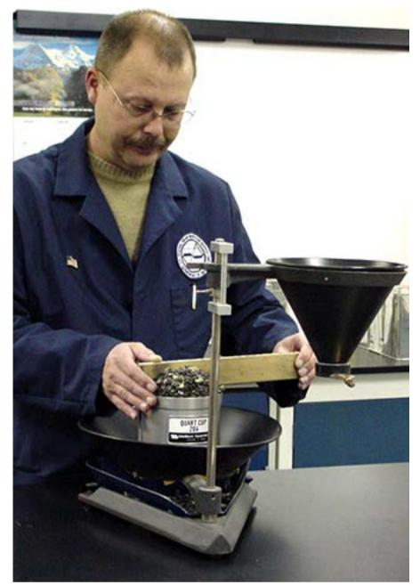
Move the kettle to a scale and record the test weight measurement.
