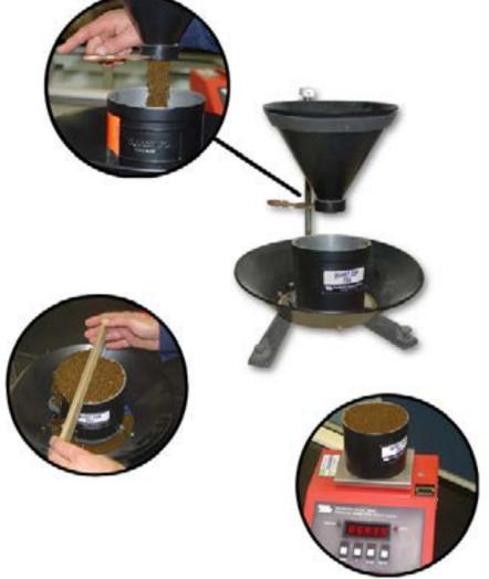
Position the hopper over the center of the kettle, making sure the hopper value is closed. Pour grain into the hopper.
