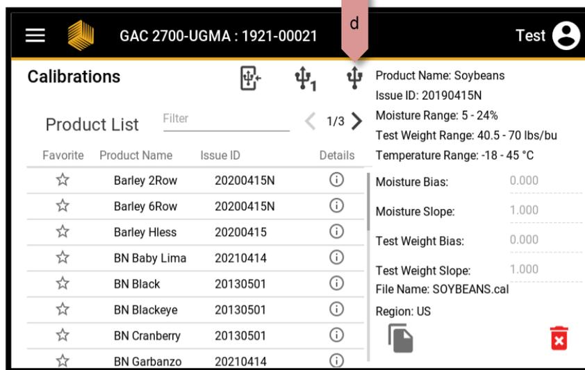
4) Press the
