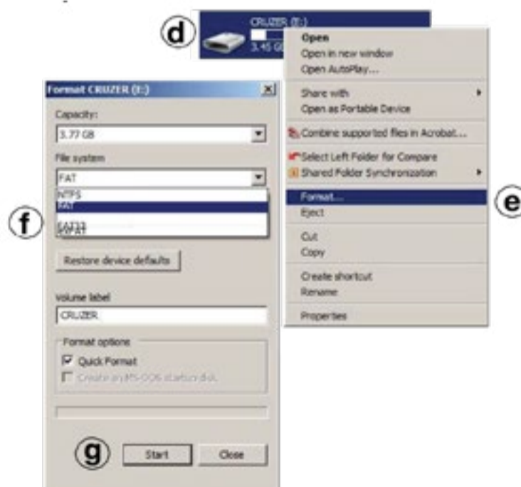
Figure 10. Formatting Memory Device to FAT
