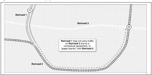
Figure 8-13: Schematic of a paper barrier
