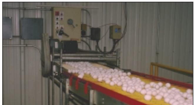
Figure 7. In-line conveyor moves eggs directly from laying houses to processing area. (CD 8202 3241 1143-72)
