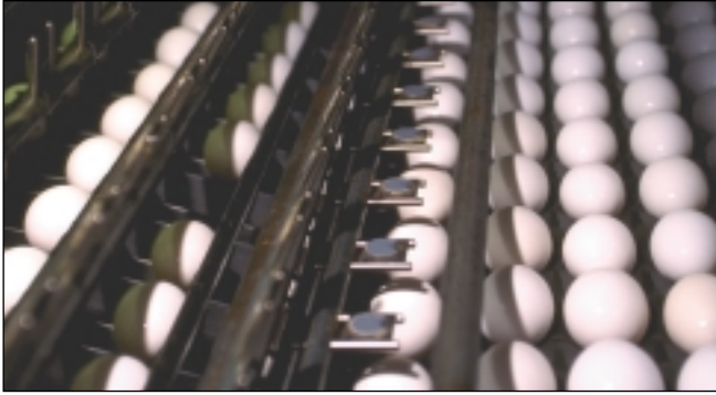
Figure 16. In-line electronic scales weigh and sort individual eggs by weight classes so that they can be diverted to the proper packaging lines. (CD 8202 3241 1143-30)
