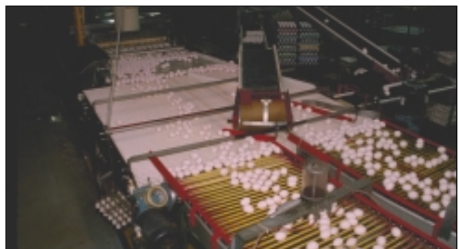
Figure 8. Eggs from multiple in-line and off-line systems are conveyed to centralized orientation area before entering washer. (CD 8202 3241 1143-80)
