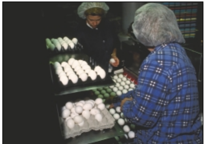
Figure 14. Plant personnel segregate broken and dirty eggs after the washing cycle and prior to the candling operation. (CD 8202 3241 1143-1)
