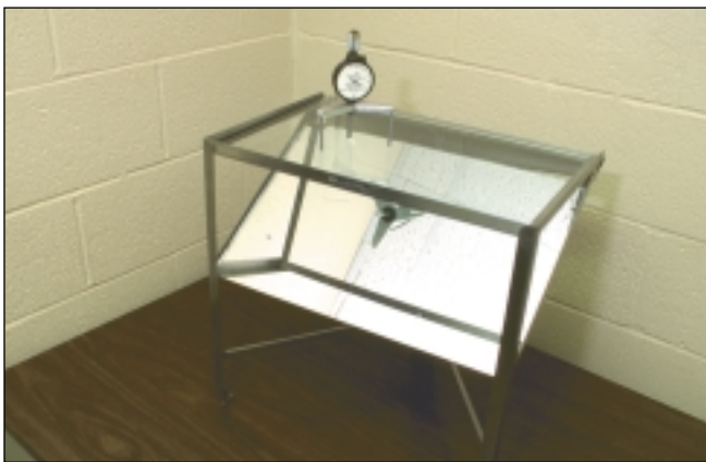
Figure 51. Egg breakouts are conducted on equipment which typically includes a metal stand, glass top, and reflective mirror. (CD 8202 3241 1143-11)
