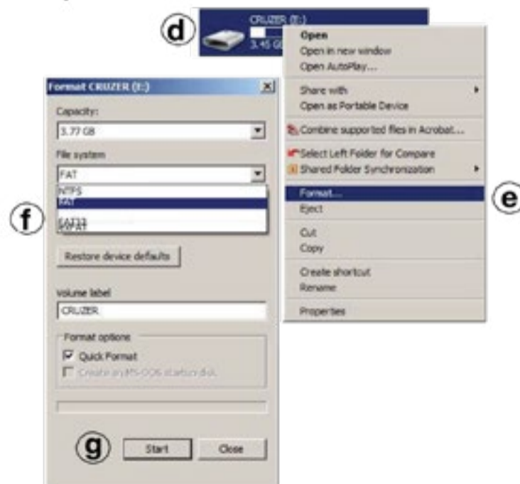
Figure 10. Formatting Memory Device to FAT
